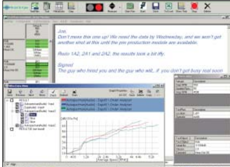
Fig. 1 A typical layout for a TestPlan running one test setup. The meta-data window is shown in the bottom, right-hand corner and the data view window with explorer is shown across the bottom. A note from the test engineer to the test operator is shown in the explorer window
